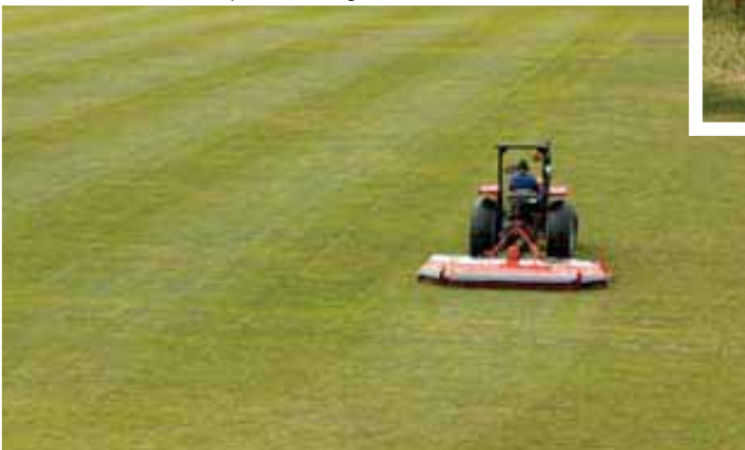
The StealthS2 can be operated with one or both wings raised, giving the added versatility of three cutting widths in one mower.
