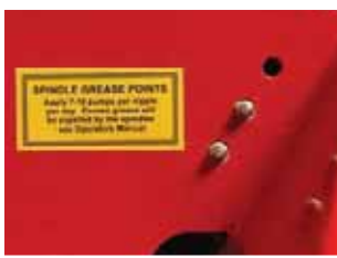
Remote grease points for hassle-free lubrication and maintenance.
