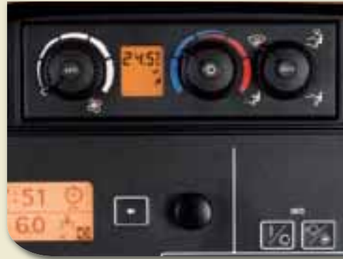
Optional Clima Track automatic temperature control allows you to specify a temperature; the system keeps it there, automatically adjusting vents and blower speeds as needed.
